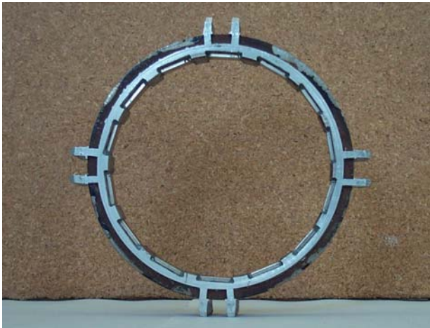
Figure 4. Fourteen pole rotor with permanent magnets.
