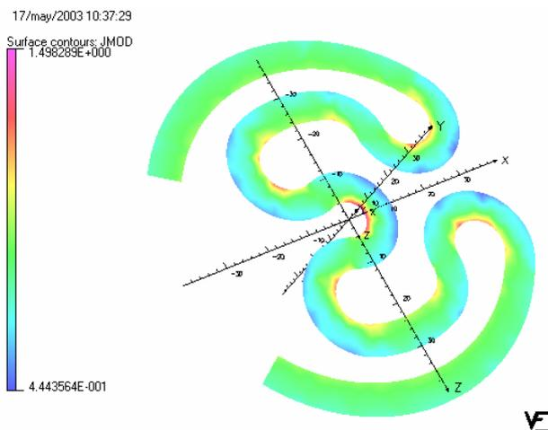
Figure 9. Module of J contour map calculated by FES.
