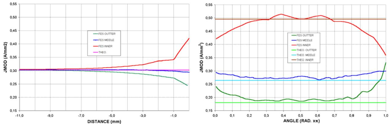
**Figure 6.** Current density along the straight and curve sections for different parallel path. (comparison between second approach and FES solutions).
