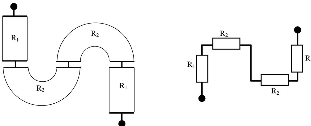
**Figure 2.** Studied resistor divided into pieces and its equivalent circuit.
