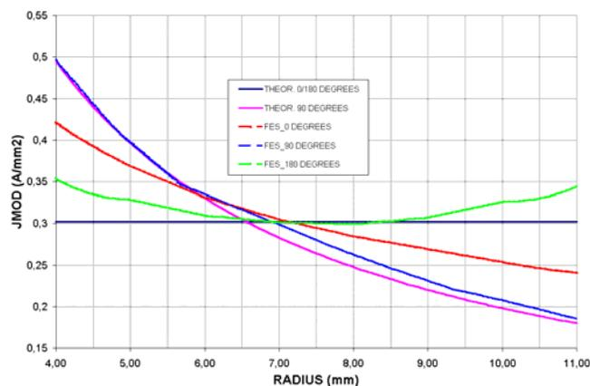
**Figure 7.** Current density along a cross-section for different angular position. (analytical and FEM solutions).
