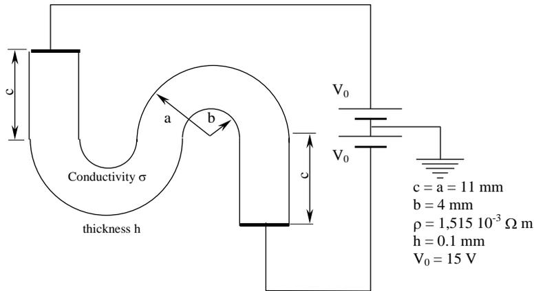
**Figure 1.** Schematic of the resistor and its connections.
