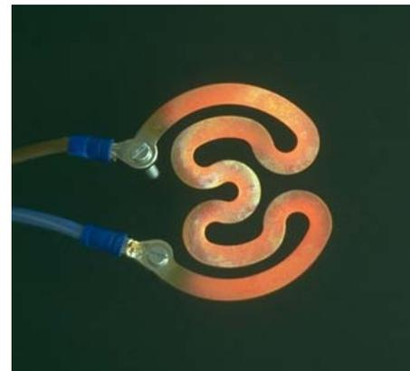
Figure 10. Thermograph map for the resistance.
