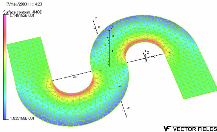
**Figure 3.** Current density distribution at the simplified piece.
