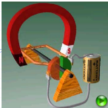
How Magnets Make a DC Motor Work This motor has a horseshoe magnet (in red) and an electromagnet (turning).
