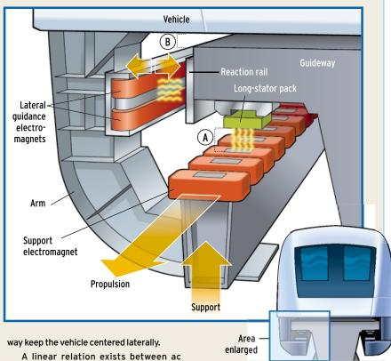
A linear relation exists between ac frequency and train velocity. At 270 Hz, for example, the vehicle would move at 500 km/h. What's more, linear generators, integrated into the levitation magnets, derive power from the traveling electromagnetic field when the vehicle is in motion. This contactless energy exchange supplies power for the on-board equipment, levitation, and battery recharging.
